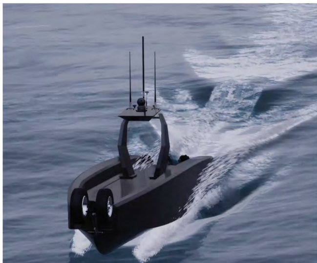
With its deep-vee planing hull, Prowler operates as a conventional surface vessel when underway.
