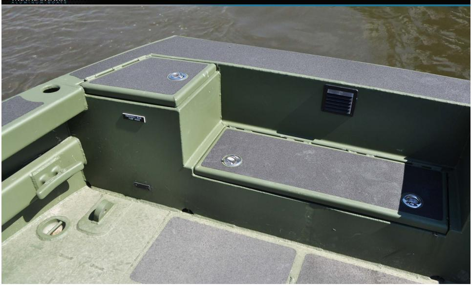
Additional Features: Integrated forward boarding step allows for quick, surefooted access during landing operations. Low-level LED lighting discretely illuminates walkways. Ample storage space can be found belowdecks.
