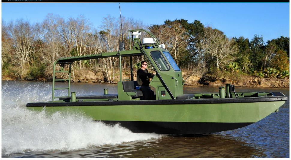
The Metal Shark 24 Riverine is rugged and reliable, with fully-welded construction and heavy-duty ¼" aluminum bottom plates providing the heft to withstand harsh operating conditions. Equipped with a dependable Yanmar 370 engine and a Hamilton 274 jet drive featuring built-in cooling and hydraulic reverse bucket technology, the 24' Riverine can perform capably in less than 18" of water.
