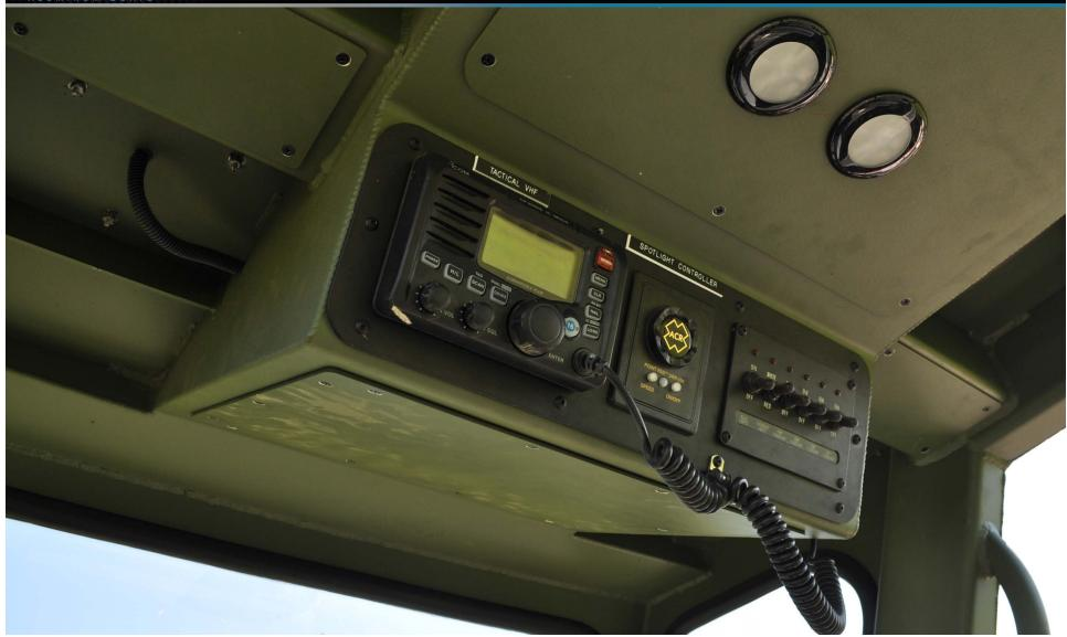
Additional Features: Communications systems, spotlight controller, and auxiliary switches are mounted in the overhead electronics pod with easy maintenance access provided. White/red overhead LED lighting is standard.
