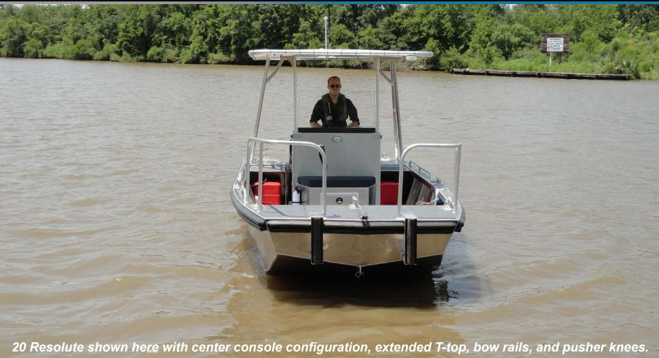
Built to Last. With their wide beams and even wider array of available configurations, Metal Shark's Resolute skiffs may be fully customized to meet the needs of the most demanding customers. Available in 30', 20', and 16', these fully-welded workhorses are made of premium quality, corrosion resistant 5086 alluminum allow and built to withstand years of use, even in the most brutal conditions.
