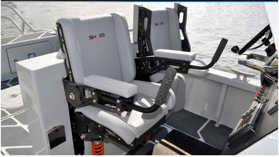
**Seating:** Many seating options are available. The 28 Relentless is shown here with side by side SHOX shock mitigating high performance seats with fold-down pistol-grip armrests and drop-out bottoms. There are numerous options available in terms of shock mitigating seats, or alternately, conventional seats or a leaning post may be installed. Customers may choose fixed second-row seating, or seats that fold away into the cockpit sole.
