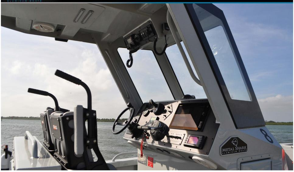
Console & Integrated Hard Top: The 28 Relentless features a welded aluminum console with integrated hard top. The hard top is available in a fold-down configuration that allows it to be quickly stowed for transport. Metal Shark's use of pillarless fritted-fit glass substantially enhances visibility by reducing dangerous blind spots.
