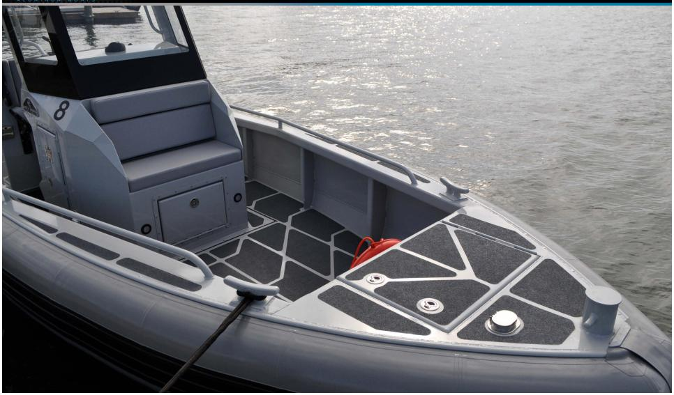
**Forward Cockpit:** The 28 Relentless features a roomy forward cockpit with non-skid cockpit sole and ample free-board. There's a large anchor locker forward, along with welded towing bit. Also shown here is the integrated console seat and backrest in the forward console.
