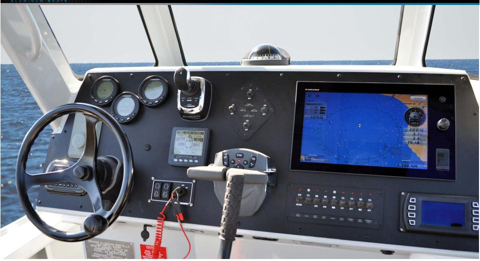
Helm: The 28 Relentless features a large dash that easily accommodates all controls and electronics, allowing for ideal placement and easy, intuitive operation. The vessel shown here is equipped with Evinrude's ICON controls, Optimus 360 joystick control system, large Furuno multifunction screen with GPS, radar, and FLIR camera. Like all Metal Sharks, the 28 Relentless is a fully custom vessel that is built to order, so the customer may determine the dash components as well as their layout.
