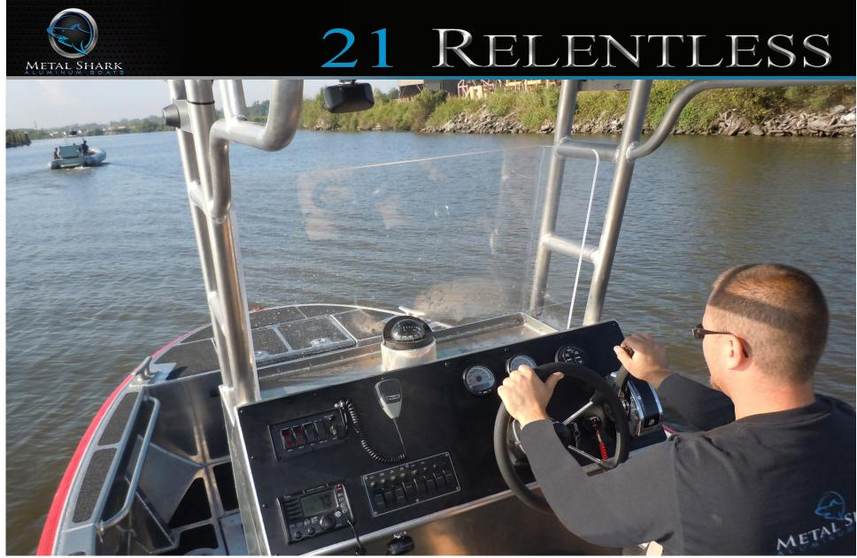
Console, Dash, & Integrated T-top: The 21 Relentless features a welded aluminum console with integrated canvas T-top and an acrylic windscreen that combine to provide protection from the elements. A large dash area easily accommodates all controls and electronics. Like all Metal Sharks, the 21 Relentless is a fully custom vessel that is built to order, so the customer may determine the dash components as well as their layout.
