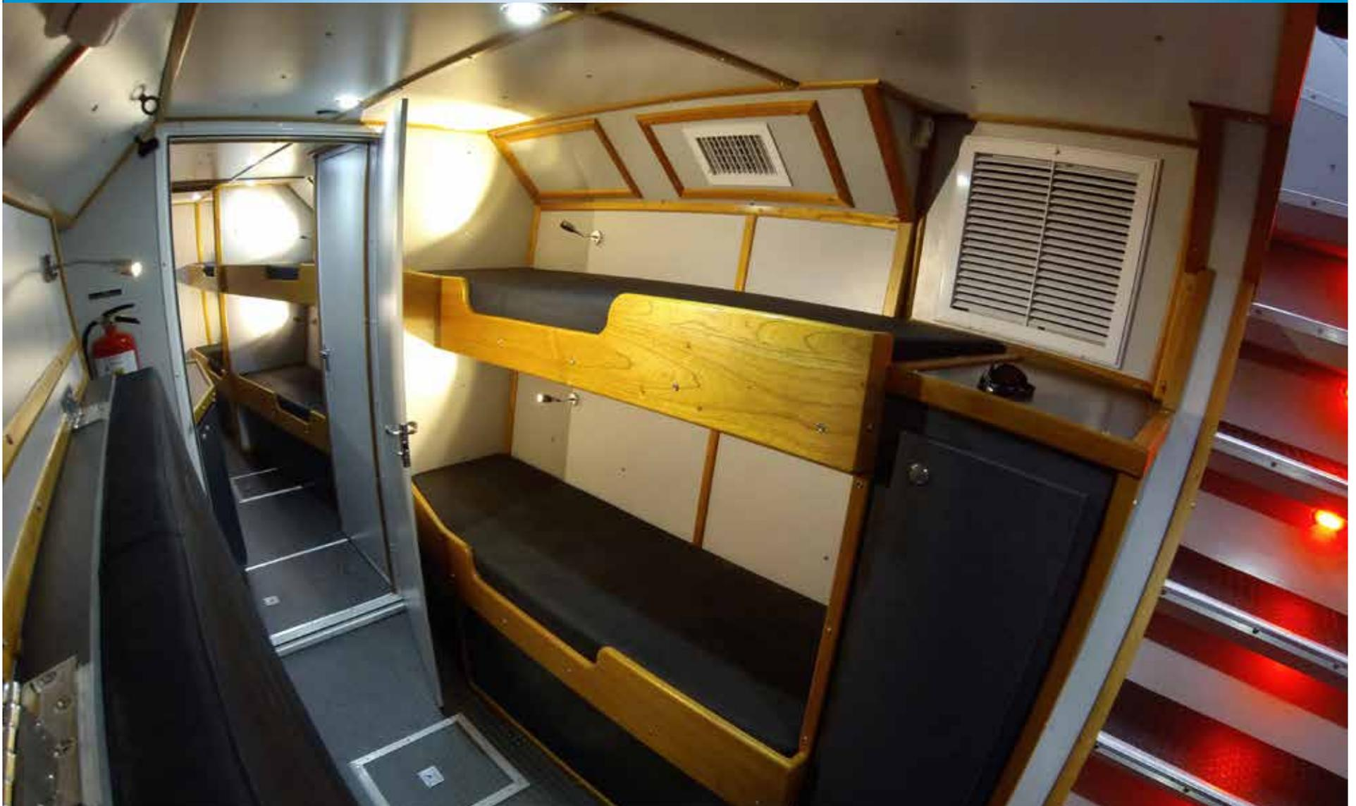
**Crew Accommodations:** Below-decks, the twin hulls provide berthing for a crew of up to twelve, with an enclosed head. Sleeping accommodations are separated from the pilothouse allowing off watch crew to rest without disrupting operations. Layouts may be modified to fit virtually any mission profile.
