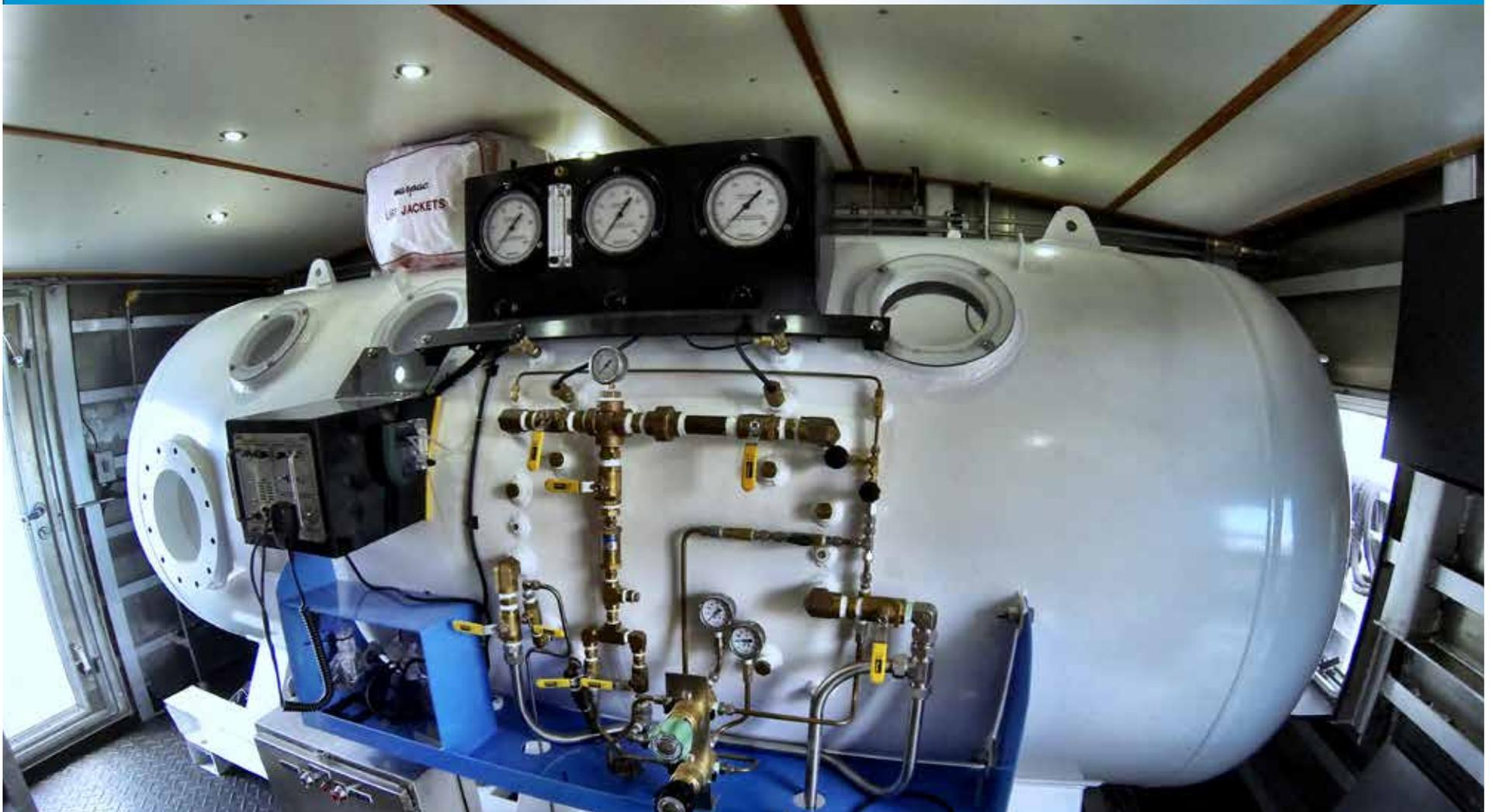
**Diveboat Capability:** The 75 Endurance may be custom-configured for a wide range of applications. Shown here is an onboard decompression chamber installed in a 75' Endurance dive boat. For dive operations the 75 Endurance can accommodate custom equipment including dive station, deck decompression chamber, Nitrox O2 enriched diving system, jet pump, 5,000lb crane, diver hydraulics, diver hot water, FLIR camera, LRAD, diver recovery system, and a deployable recovery RIB.
