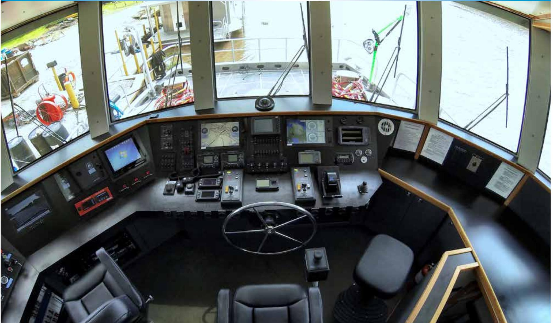
**Helm:** The 75 Endurance DSV features a massive dash area that easily accommodates all controls, instruments, and navigation equipment, allowing for easy operation of the vessel and all onboard systems. The elevated helm affords an outstanding view; facilitating navigation and maneuvering during multi-vessel maneuvering or dive ops.
