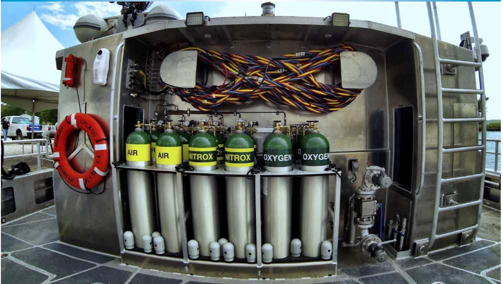
**Diveboat Capability:** Shown here is the aft deck dive station of a 75 Endurance DSV. For dive operations the 75 Endurance can accommodate custom equipment including dive station, deck decompression chamber, Nitrox O2 enriched diving system, jet pump, 5,000lb crane, diver hydraulics, diver hot water, FLIR camera, LRAD, diver recovery system, and a deployable recovery RIB.
