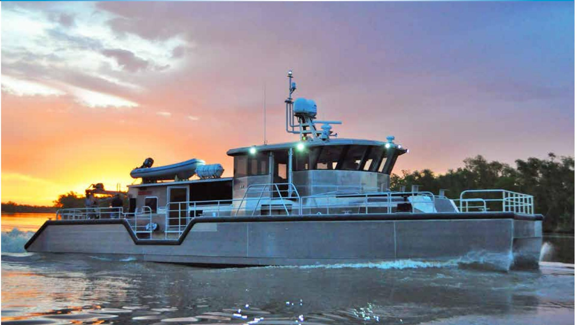
The **Metal Shark 75 Endurance DSV** is a welded aluminum pilothouse catamaran specially designed for dive support operations. Its wide beam affords ample stability, and its roomy belowdecks accommodations allow crews to remain at sea for extended periods. Like all Metal Sharks, the 75 Endurance DSV may be fully customized to meet a wide range of specialized mission requirements.
