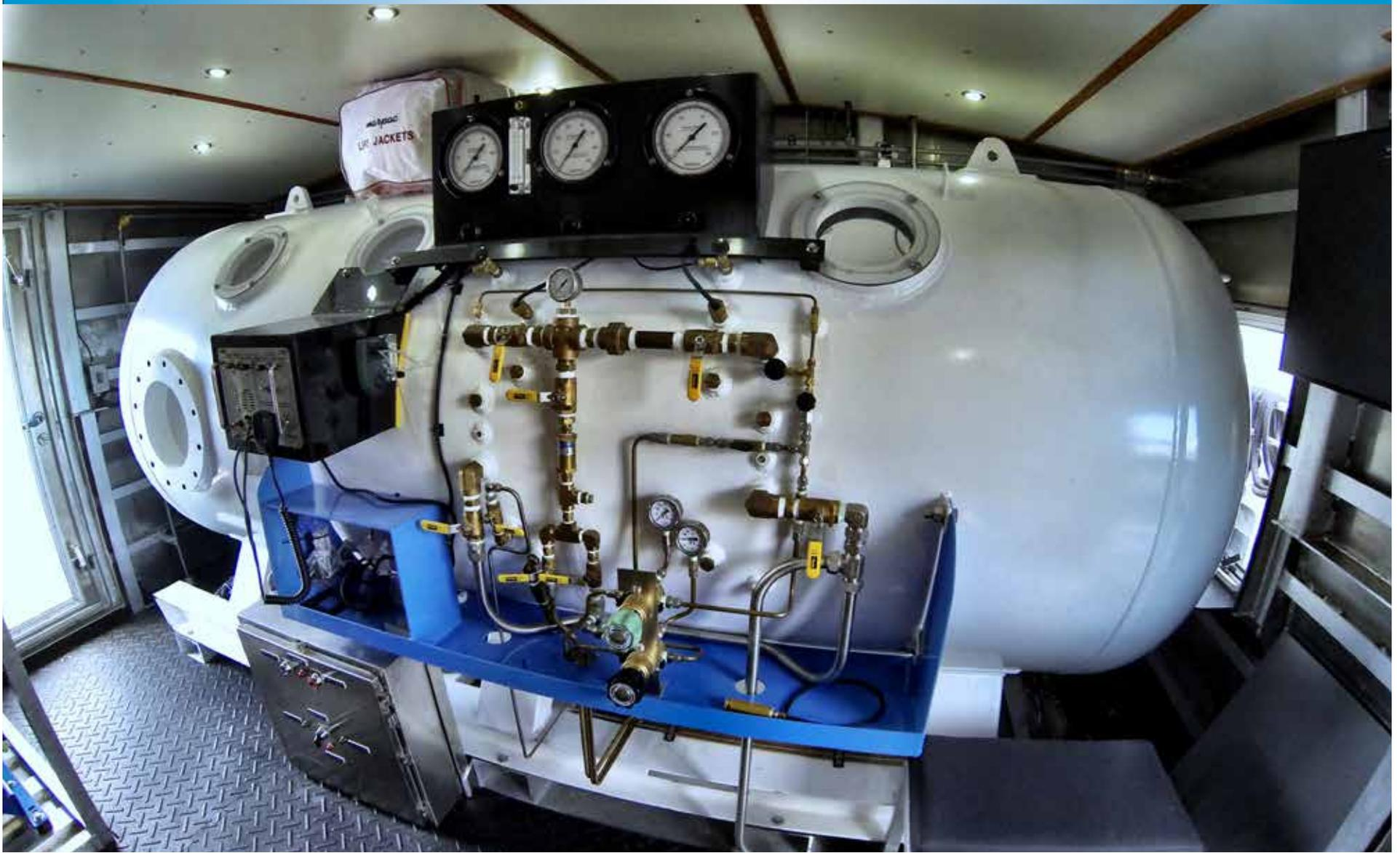
**Diveboat Capability:** Shown here is an onboard decompression chamber installed aboard a 75 Endurance DSV. With its spacious layout, the 75 Endurance DSV easily and capably accommodates complex onboard systems.
