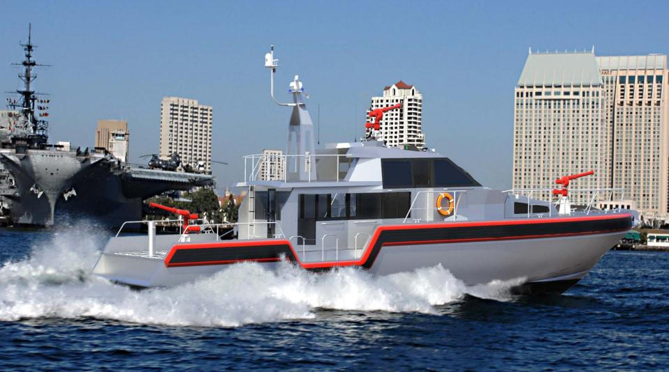
Hull Design: The 75 Defiant features a proven Metal Shark hull design that has been engineered and built to precise tolerances. To achieve its superior hull life rating of 30+ years, the vessel's hull, deck, and pilothouse structure are composed entirely of heavy, welded plates of premium-grade 5086 aluminum alloy. Thanks to its wide 21' beam, the 75 Defiant is extremely stable yet surprisingly fast, capable of speeds in excess of 40 knots.
