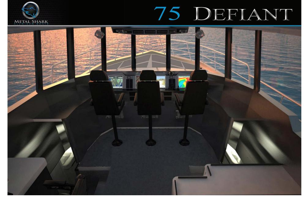
Helm: The 75 Defiant helm features a massive dash area that easily accommodates all controls, instruments, and navigation equipment, allowing for easy operation of the vessel and all onboard systems. The elevated helm affords an outstanding view; facilitating navigation and maneurvering in multi-vessel and/or fire fighting operations.
