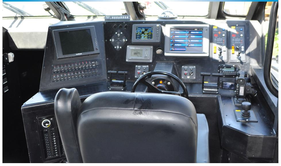
Helm: The 64 Defiant features a massive dash area that easily accommodates all controls, instruments, and navigation equipment, allowing for easy operation of the vessel and all onboard systems. The elevated helm affords an outstanding view; facilitating navigation and maneurvering in multi-vessel and/or fire fighting operations.
