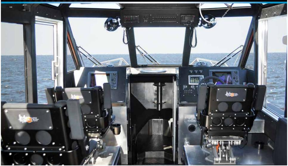
Helm: Inside the pilothouse, the entire crew benefits from the massive windows, overhead skylights, and large opening side and aft doors. Self-parking windshield wipers and window defrosters maintain visibility during inclement weather. The spacious port and starboard helm areas easily accommodate a wide array of custom-installed electronics, with additional mounting space available in the overhead electronics pod.
