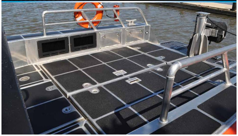
Aft Cockpit: The 38 Defiant boasts a massive, wide-open working deck, with ample room for backboards or other equipment. Large in-floor hatches open to reveal the 38 Defiant's massive engine compartment, and gasketed dry storage lockers have been provided to port and starboard. Other notable features shown here include the optional machine gun mount and towing bit, line spool, and tubular aluminum swim platform with dive ladder.
