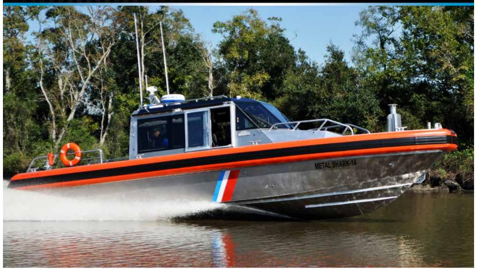
The Metal Shark 38' Defiant is a welded aluminum monohull pilothouse patrol vessel specially designed for use as a law enforcement, port security, and military patrol boat. Like all Metal Sharks, it may be fully customized to meet virtually any mission requirement. Regardless of configuration and equipment, the 38' Defiant serves as an extremely stable, dependable, and highly capable platform that is well suited for both inland and offshore use.
