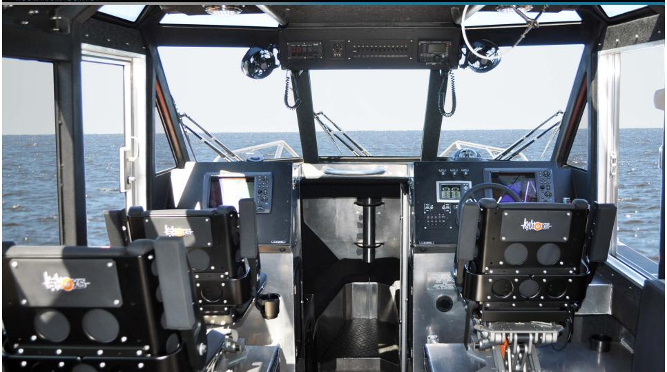
Helm: Inside the pilothouse, the entire crew benefits from the massive windows, overhead skylights, and large opening side and aft doors. Self-parking windshield wipers and window defrosters maintain visibility during inclement weather. The spacious port and starboard helm areas easily accommodate a wide array of custom-installed electronics, with additional mounting space available in the overhead electronics pod.
