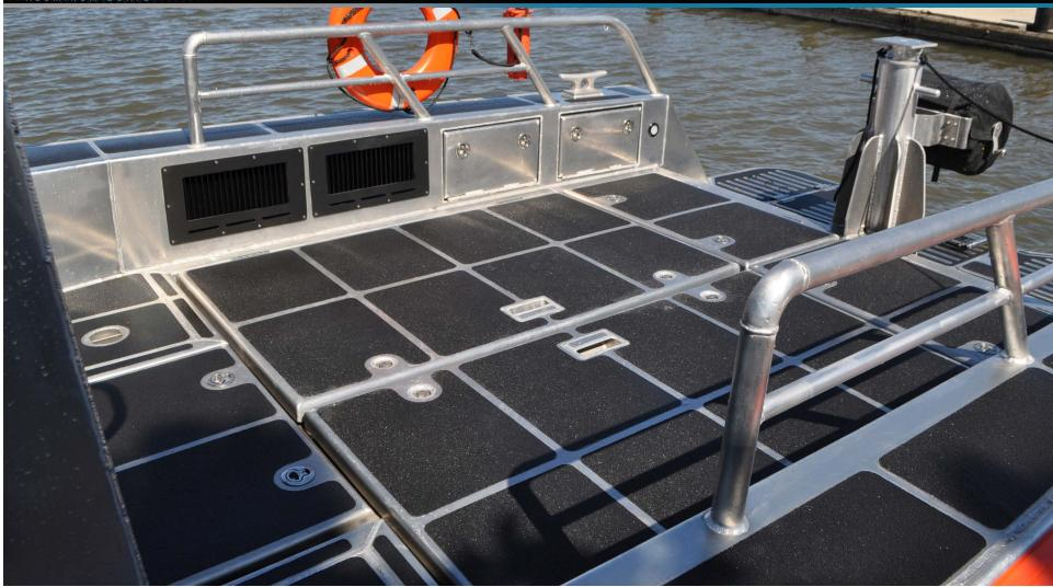
Aft Cockpit: The 38 Defiant boasts a massive, wide-open working deck, with ample room for backboards or other equipment. Large in-floor hatches open to reveal the 38 Defiant's massive engine compartment, and gasketed dry storage lockers have been provided to port and starboard. Other notable features shown here include the optional machine gun mount and towing bit, line spool, and tubular aluminum swim platform with dive ladder.
