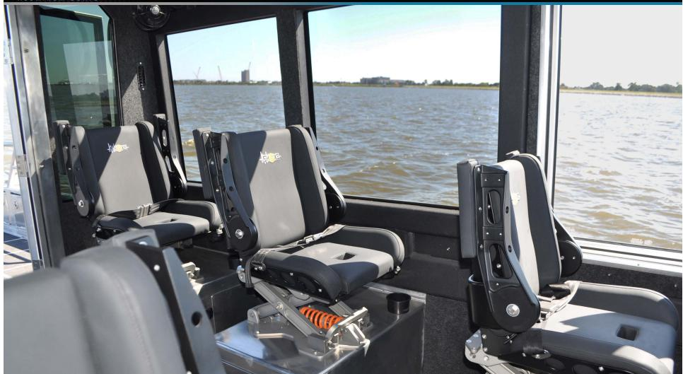
**Seating:** The 38 Defiant is shown here in a water ambulance configuration: Three shock-mitigating seats are located on the port side, with another at the starboard helm just ahead of a bench seat that converts to twin bunks. There are latching storage compartments beneath each seat, and well-placed grab rails throughout. Numerous seating options and available climate control combine to afford a high level of crew comfort regardless of the mission at hand.
