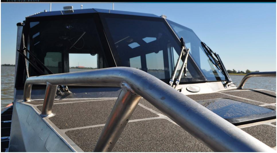
Pilothouse: The 38 Defiant's spacious pilothouse provides all-weather comfort and security for the entire crew, and thanks to Metal Shark's implementation of pillarless glass technology, it also offers best-in-class safety and visibility. Metal Shark implemented this design in order to significantly reduce the dangerous blind spots that are so prevalent in conventional pilothouse vessels, and the results are immediately apparent upon stepping aboard.
