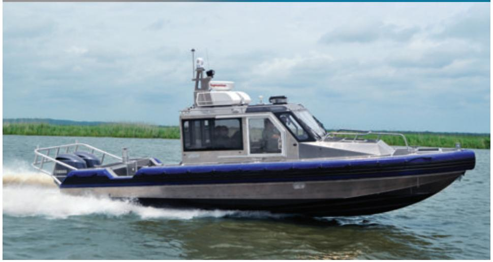
Hull Design: The 32' Defiant features a proven Metal Shark hull design that has been engineered and built to precise tolerances. To achieve its superior hull life rating of 30+ years, the hull is composed entirely of heavy, welded plates of premium-grade 5086 aluminum alloy. Thanks to its wide beam and pronounced revervse chines, the 32' Defiant is extremely stable, and twin 300 HP outboard engines require minumum maintenance while reliably propelling the vessel to speeds in excess of 45 knots.
