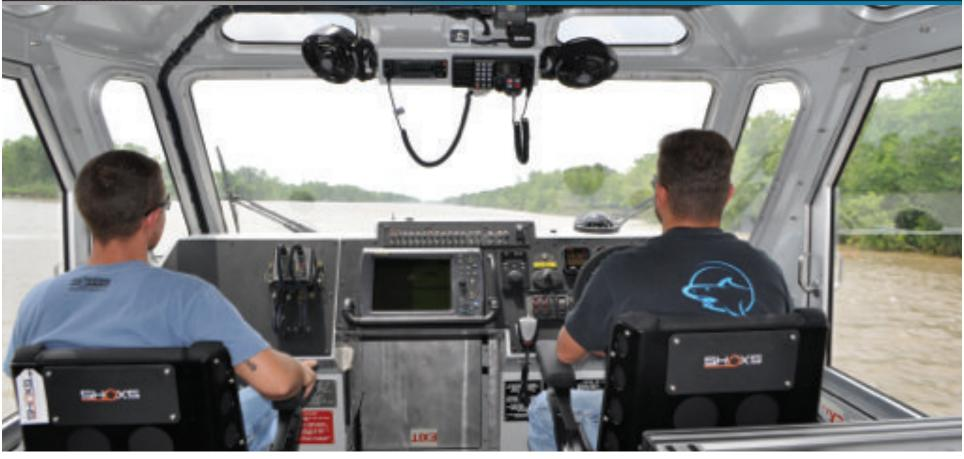
**Pilothouse:** The most immediately apparent advancement in Metal Shark's Defiant pilothouse design is the use of pillarless glass to substantially enhance visibility (please note that the vessel shown here has been built to U.S. Navy specs, with mechanically fastened windshield glass in lieu of our Diamond Seaglaze fritted glass). The result is a near elimination of the dangerous blind spots that are an unfortunate drawback of conventional pilothouse vessels. Further,
