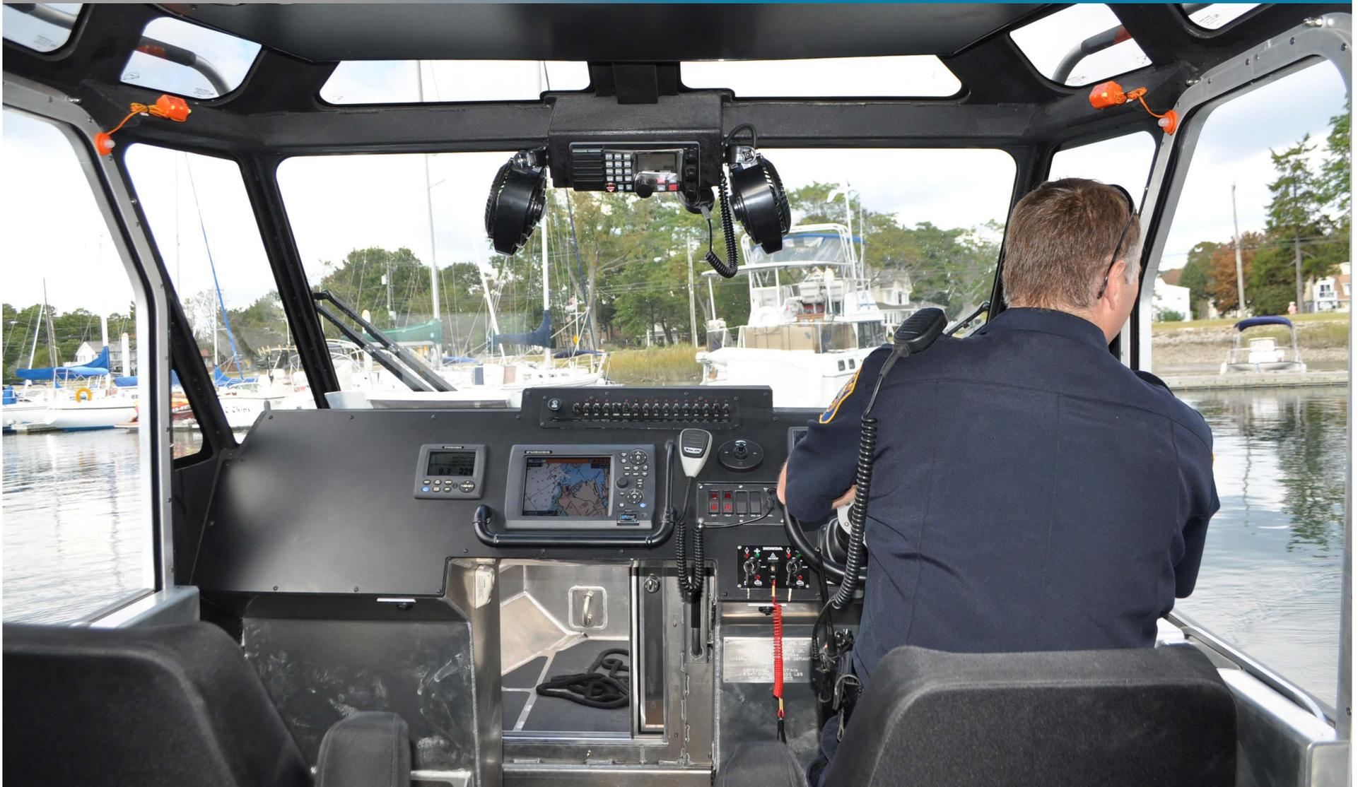
**Pilothouse Design:** The most immediately apparent advancement in Metal Shark's Defiant class is the use of pillar-less glass to substantially enhance visibility. The result is a near elimination of the dangerous blind spots which are an unfortunate drawback of conventional pilothouse vessels.
