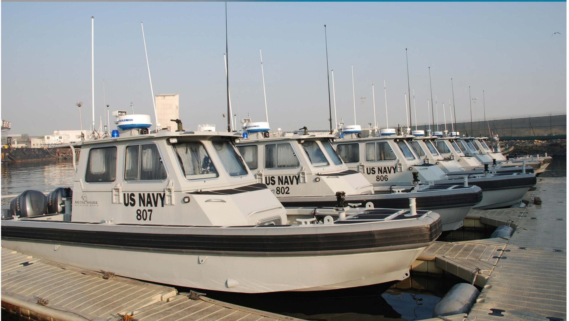
**Choice of the US Navy.** The Metal Shark 27 Defiant currently serves as the US Navy Force Protection Boat – Small. In FPB-S configuration, the 27 Defiant features a more conventional windshield, but offers the advantage of a convertible pilothouse that folds down and stows away for transport.
