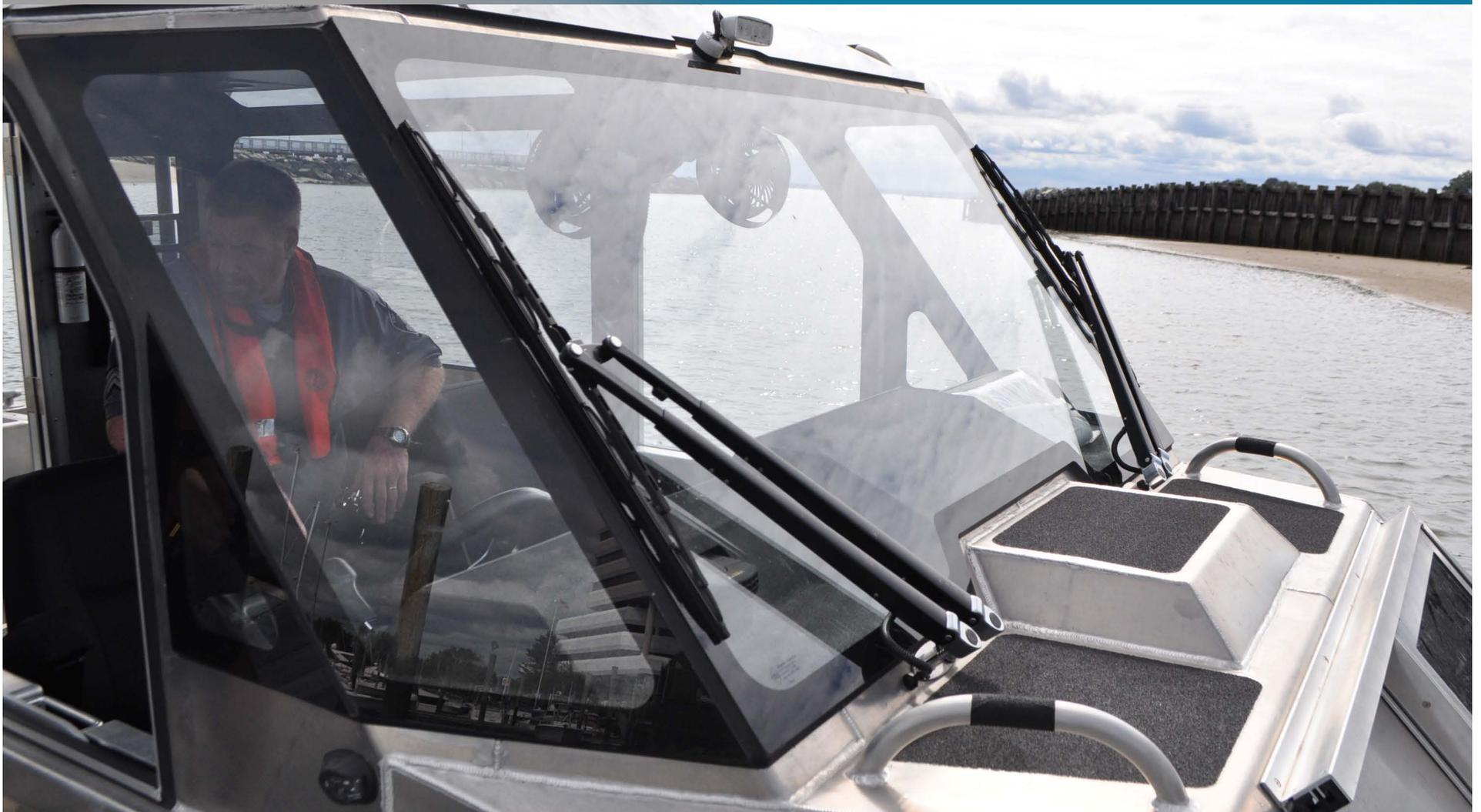
**Windshield:** The 27 Defiant's front windshield is composed of a single piece of glass, with no center pillar to obstruct the view from the helm. This, coupled with the overall height of the windshield and windows, overhead spotter lights, and large side and aft opening doors, combine to provide an unprecedented level of visibility. The end result is a vessel that is substantially easier to operate, especially during inclement weather or night missions.
