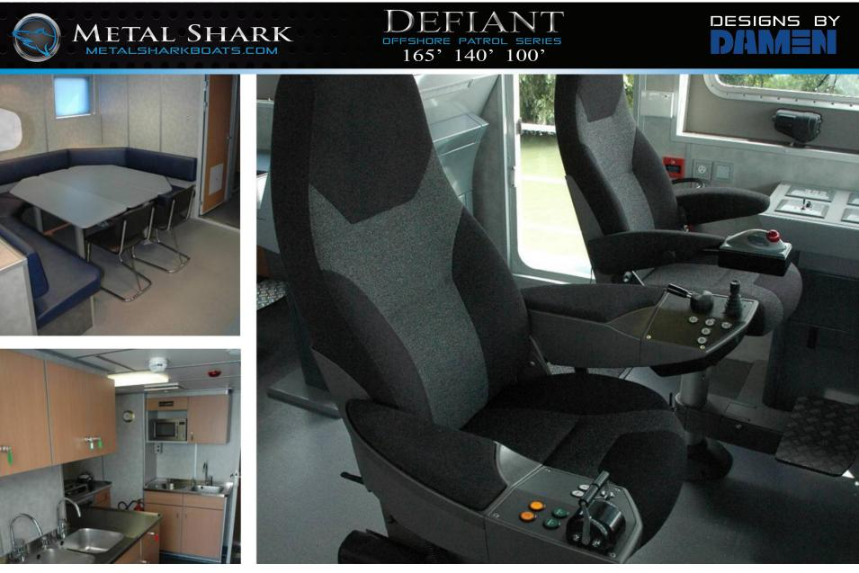
Crew Ergonomics: The major controls and communication devices of each Defiant Offshore Patrol vessel are integrated into the helmsman's seat. Even in the most inclement conditions, the helmsman can easily and comfortably control the ship. Throughout the vessel, flexible carpentry and floating floors have been deployed to reduce vibration. Like all Metal Sharks, interior layout may be fully customized to suit virtually any mission requirement.
