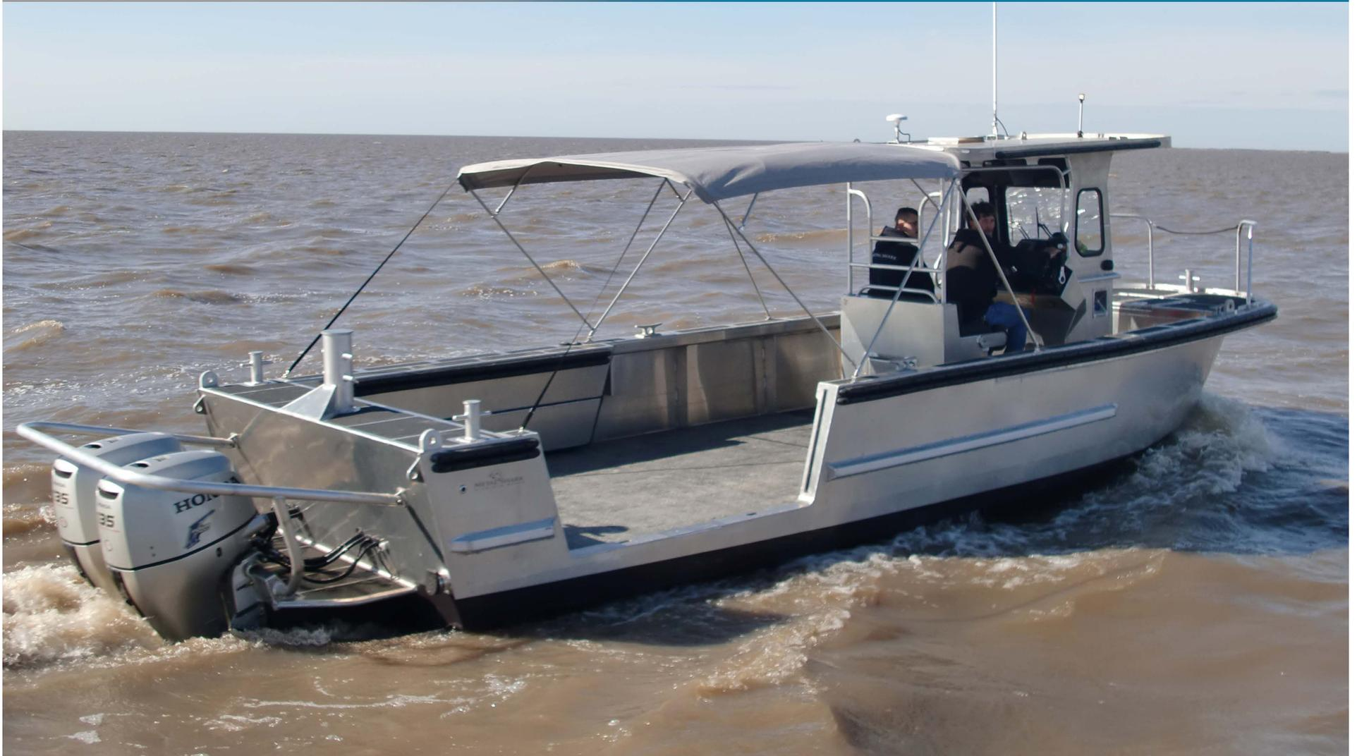
**Available Forward-Console Layout:** The 28 Courageous is available in an alternate configuration with a forward console and massive aft cockpit. Also available and shown above are a two-part removable dive door measuring nearly 7' long, and a Bimini top extension that works in conjunction with the vessel's hard top to provide a large shaded area for crew and/or payload.
