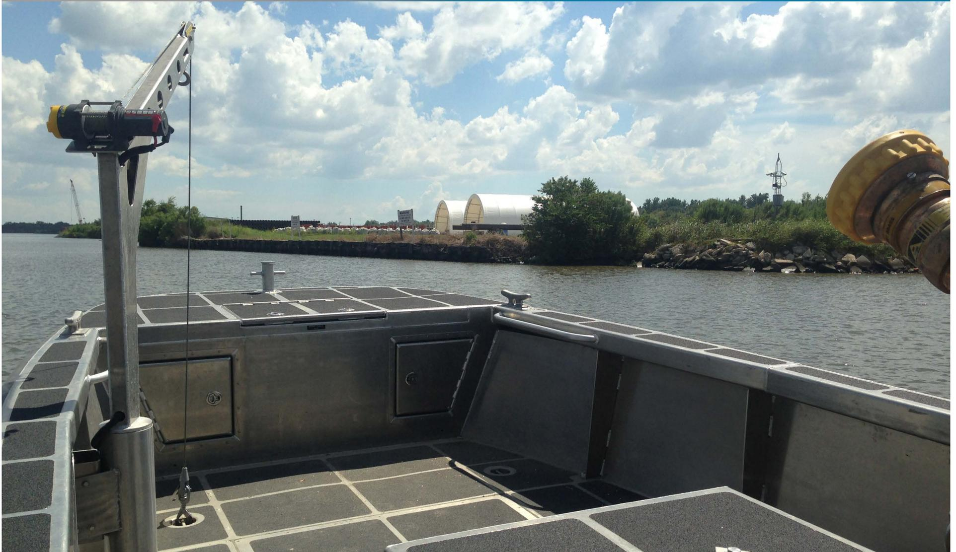
**Deck Layout:** Thanks to its flared bow, wide reversed chines, and 10' beam, the 28 Courageous is extraordinarily stable and dry, with a large roomy cockpit. The vessel features a massive foredeck with ample freeboard, which serves as an ideal working platform. An optional 500-750 lbs capacity removable electric davit adds extra utility.
