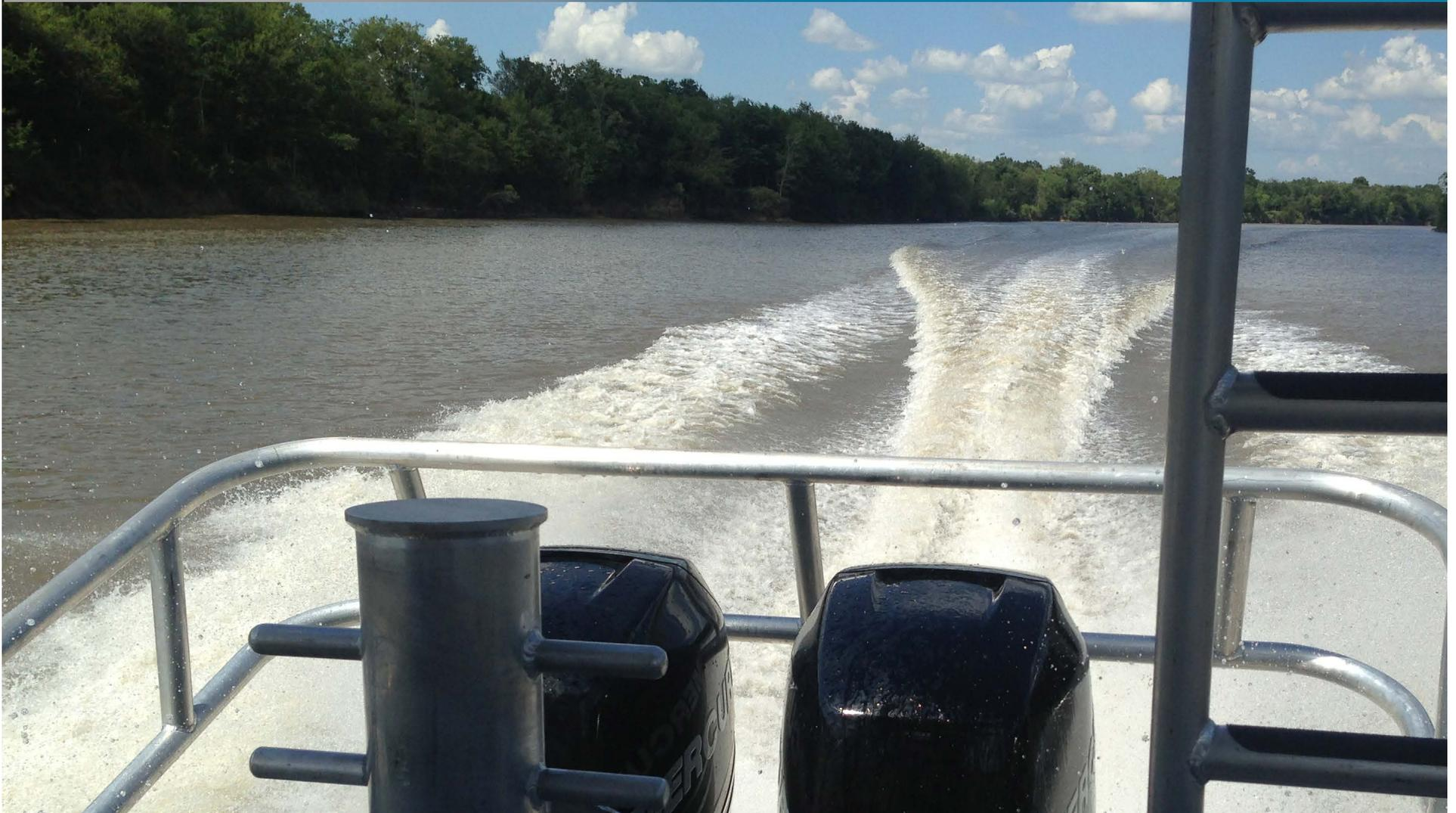
**Outstanding Performance:** With twin outboard power, the Metal Shark 28 Courageous planes quickly and features responsive handling. Top speed when powered by twin 250-horsepower four stroke outboards is in excess of 45 knots. Metal Shark is an OEM supplier for all major outboard brands and can rig according to your preference or fleet commonality requirements.
