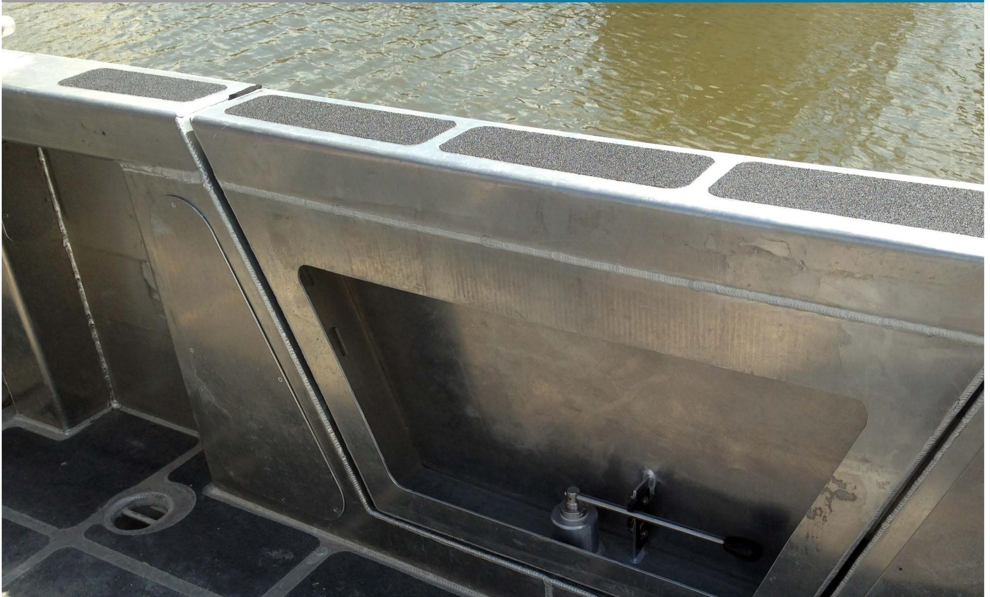
**Available Dive Door:** This large, removable door greatly facilitates water entry, especially considering the vessel's ample forward freeboard. The door latches securely in place when not in use.
