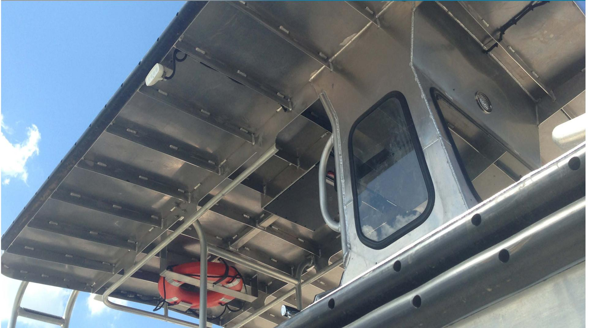
**Extended Hard Top:** The 28 Courageous is available with an extended hard top that covers the entire aft cockpit, providing shelter during rescue/recovery missions. Aft-mounted ladders provide easy access to the top's non-skid coated working surface, where removable rails allow a crew to work alongside elevated structures. A short T-top, Bimini top, full canvas enclosure, and other top options are available.
