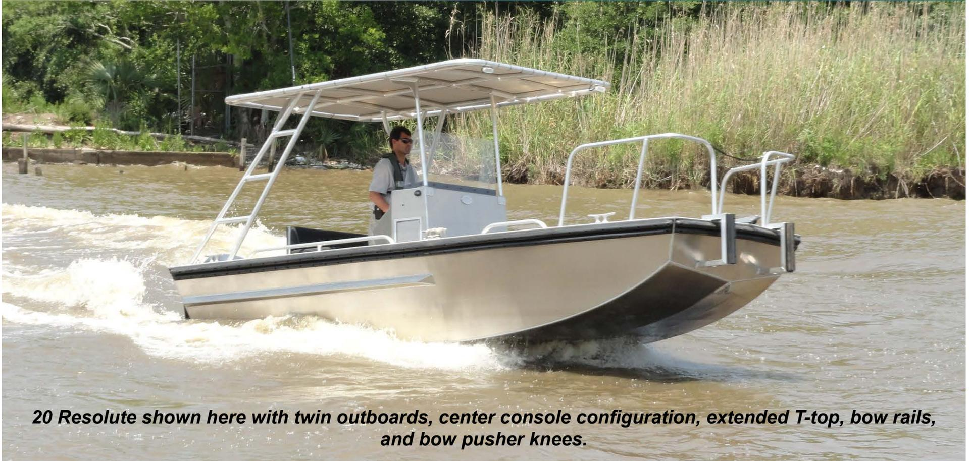
*20 Resolute shown here with twin outboards, center console configuration, extended T-top, bow rails, and bow pusher knees.*
