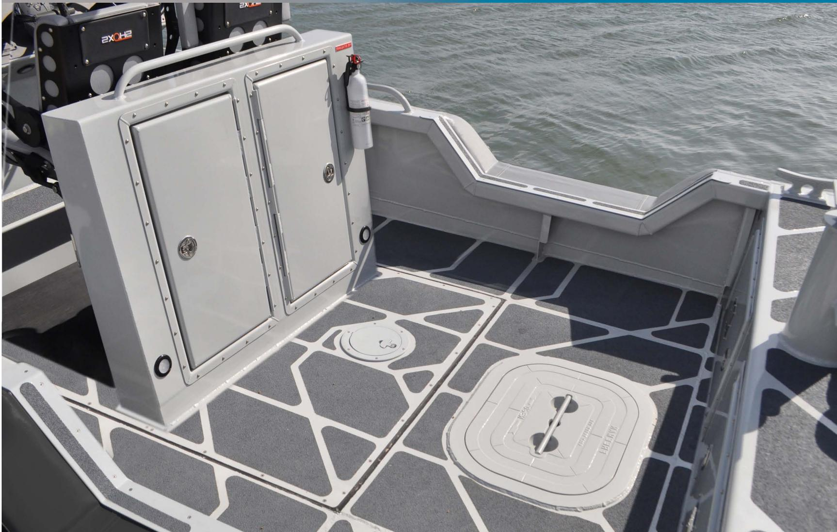
**Spacious Aft Deck:** The 26 Relentless features an uncluttered aft deck with a non-skid floor, and port/starboard dive reliefs that facilitate boarding or dive operations. (Outboard version only). Large welded cleats, towing post with line spool, and engine protection bar provide added utility. Helm seat gun locker also shown here.
