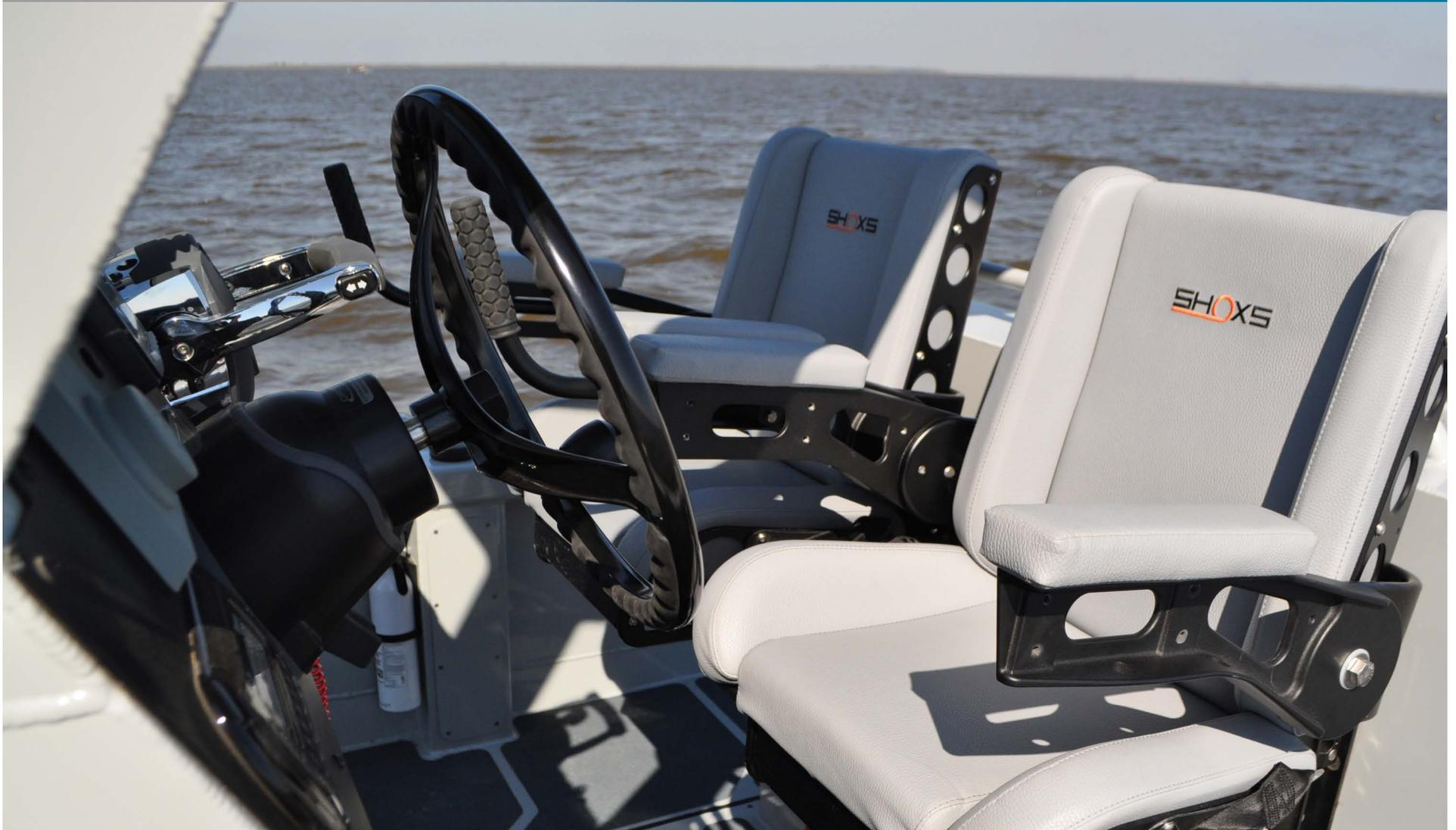
**Seating:** The 26 Relentless is shown here with side by side SHOX shock-mitigating high performance seats with fold-down pistol-grip armrests and drop-out bottoms. There are numerous options available in terms of shock mitigating seats, or alternately, conventional seats or a leaning post may be installed.
