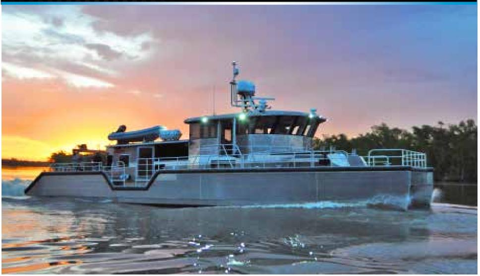
The Metal Shark 75 Endurance is a welded aluminum pilothouse catamaran specially designed for use as a law enforcement, port security, and fire rescue response boat. Like all Metal Sharks, it may be fully customized to meet virtually any mission requirement. Regardless of configuration and equipment, the 75 Endurance serves as an extremely stable, dependable, and highly capable platform that is well suited for both inland and offshore use.
