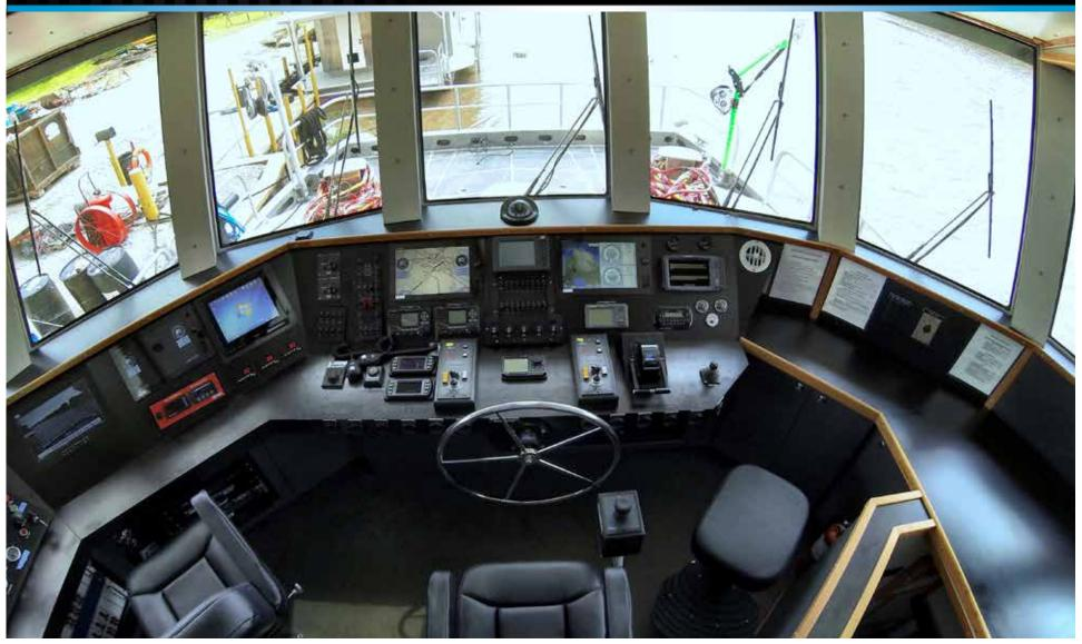
Helm: The 75 Endurance DSV features a massive dash area that easily accommodates all controls, instruments, and navigation equipment, allowing for easy operation of the vessel and all onboard systems. The elevated helm affords an outstanding view; facilitating navigation and maneurvering during multi-vessel maneuvering or dive ops.
