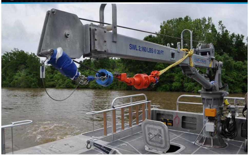
Diveboat Capability: The 75 Endurance DSV may be equipped with a large aft deck crane, such as the 2,160lb. capacity unit shown here.
