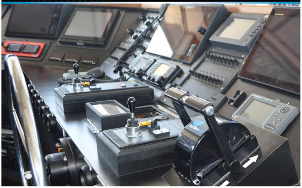
Helm Detail: The Metal 75 Endurance DSV's spacious helm can easily accommodate a full range of controls, instrumentation, navigation electronics, and specialized equipment.
