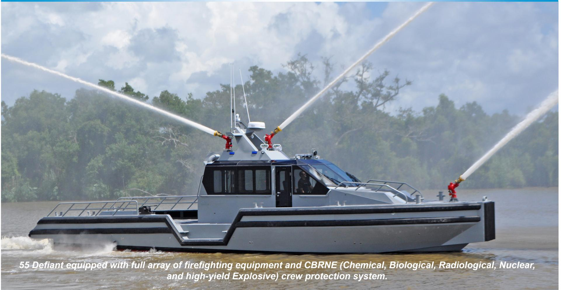
*55 Defiant equipped with full array of firefighting equipment and CBRNE (Chemical, Biological, Radiological, Nuclear, and high-yield Explosive) crew protection system.*
