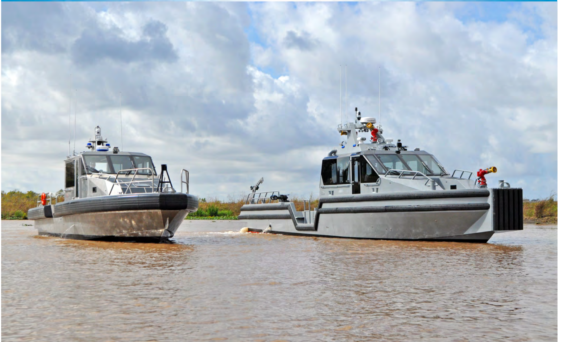
Side by side comparison shot of Metal Shark 45 Defiant (patrol configuration) and 55 Defiant (port security / fire rescue configuration).
