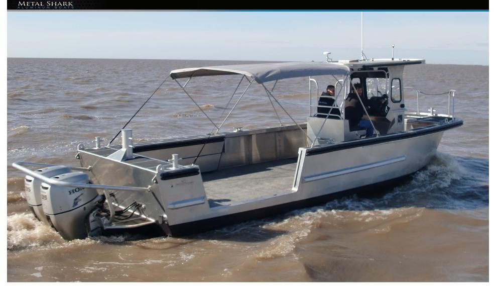
Available Forward-Console Layout: The 28 Courageous is available in an alternate configuration with a forward console and massive aft cockpit. Also available and shown above are a two-part removable dive door measuring nearly 7' long, and a Bimini top extension that works in conjunction with the vessel's hard top to provide a large shaded area for crew and/or payload.
