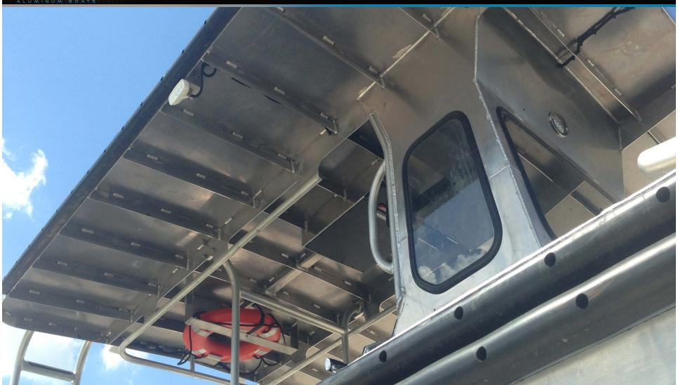
**Extended Hard Top:** The 28 Courageous is available with an extended hard top that covers the entire aft cockpit, providing shelter during rescue/recovery missions. Aft-mounted ladders provide easy access to the top's non-skid coated working surface, where removable rails allow a crew to work alongside elevated structures. A short T-top, Bimini top, full canvas enclosure, and other top options are available.
