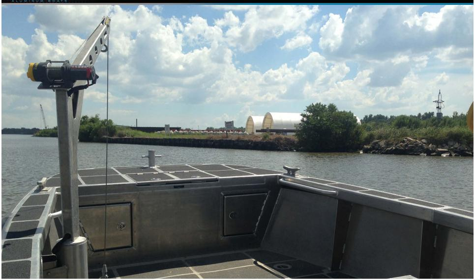
**Deck Layout:** Thanks to its flared bow, wide reversed chines, and 10' beam, the 28 Courageous is extraordinarily stable and dry, with a large roomy cockpit that is well-suited to rescue missions. Shown here with an electric davit with 500-750 lbs capacity and port-side removable dive door, the 28 courageous serves as an ideal working platform.
