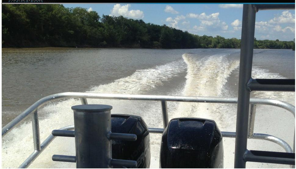
Outstanding Performance: With twin outboard power, the Metal Shark 28 Courageous planes quickly and features responsive handling. Top speed when powered by twin 250-horsepower four stroke outboards is in excess of 45 knots. Metal Shark is an OEM supplier for all major outboard brands and can rig according to your preference or fleet commonality requirements.
